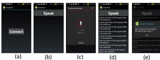
Figure 2. (a) User connects to robot. (b) User chooses to speak into phone. (c) User speaks into phone. (d) Phone displays the possible transcriptions to user. (e) Phone prompts user to send selected transcription to the robot.
